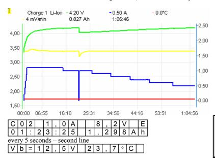
Charging ends when threshold voltage is detected and simultaneously charging current is decreased. When Fast mode is on charging current is controlled with pulses, which makes it possible to reduce charging time more than two times. Current limitation can occur when voltage
