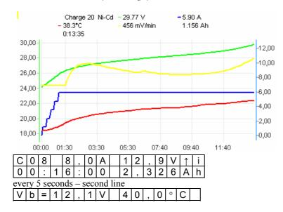
Charging ends when voltage drop  $(-\Delta v)$  or inflex point is detected. The *Inflex* mode allows finishing charging
