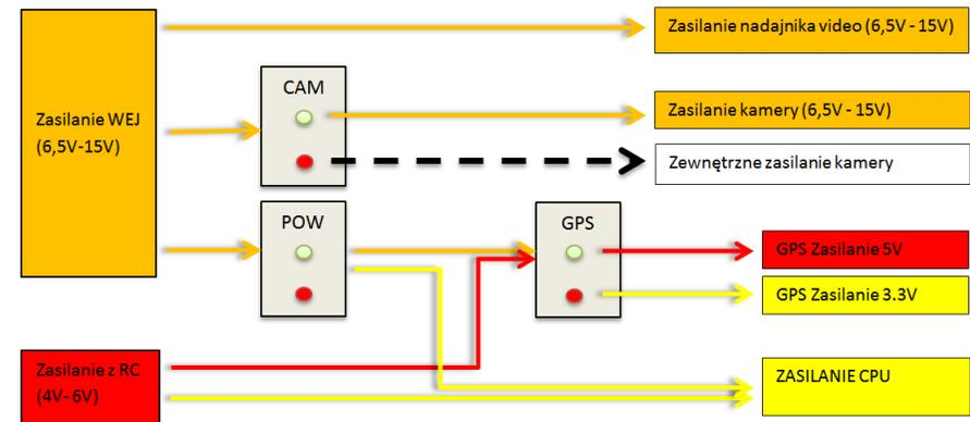
The diagram shows the OSD power supplies: INPUT (6.6 V-15V) power from RC connector (4V-6V) and CAM, POW, GPS jumpers, together with an indication of the current flow to the connectors of the external devices.
