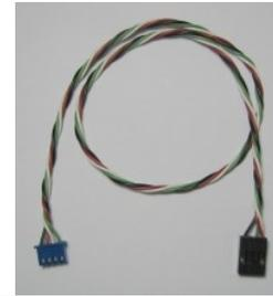
45 cm cable to connect te OSD to GPS module.
