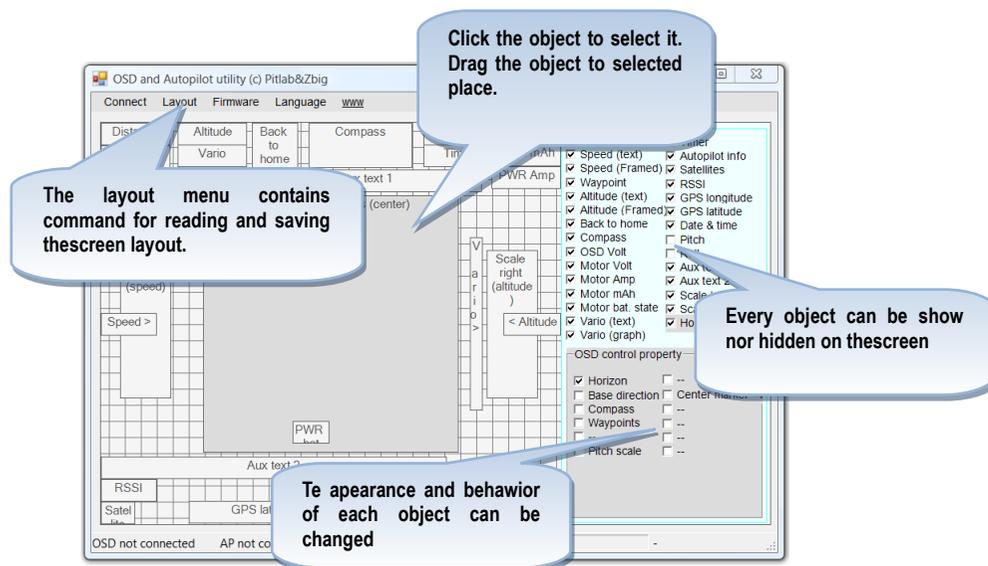
Figure 7: OSD configurator main screen.
