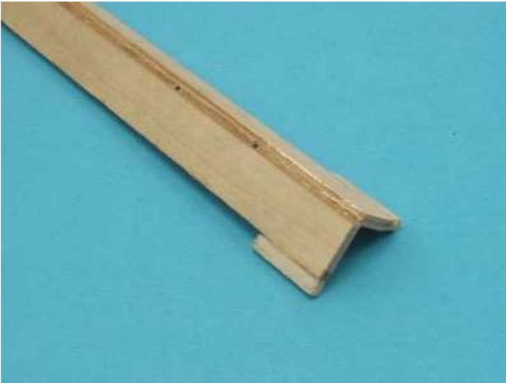
Simple jig of 3 mm ply to drill the holes for pegs 1,5 mm.
