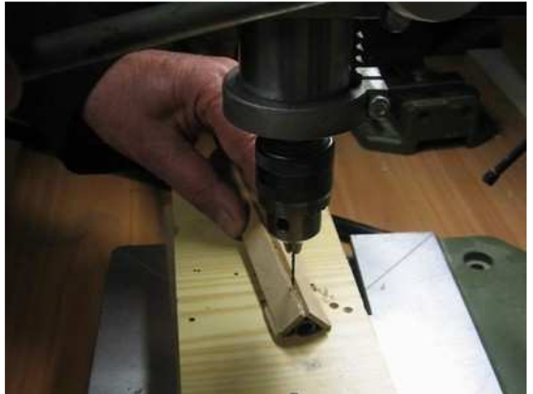
Drill 4 holes perfectly in line. Drill one hole, insert peg 1,5 mm to assure the holes are parallel and drill another 3 holes.
