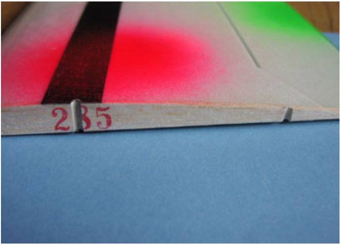
File out small notches. Check for correct location.
